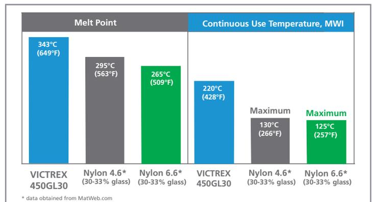
VICTREX PEEK 450GL30 valve components outperform 30% glass reinforced nylon mainly due to:
